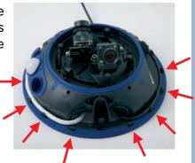
Lead cables properly through the cable guides
