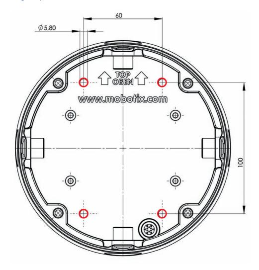
Find the drilling templates (scale 1:1) at the end of the manual as a fold-out
