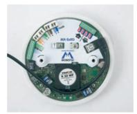
Insert USB plug Properly guide the cable
