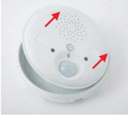
Remove the back of the housing
