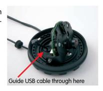
3) Insert the Mini USB plug into the Mini USB/ MOBOTIX Bus connector at the front of the lens mount. Make sure that you do not insert the plug into the audio connector by accident.
