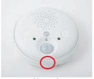
Assemble ExtlO housing Align arrows
