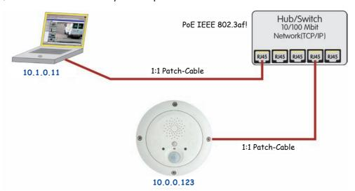
PoE switch/router according to IEEE 802.3af required
