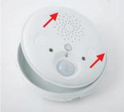
Remove the back of the housing
