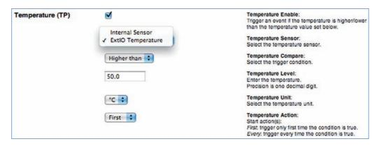
To see a table with the latest temperatures of both the ExtlO's and the camera's temperature sensor, open **Admin Menu > Temperatures**.
