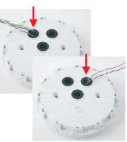
Push each wire through one of the openings of the 8-wire plug
