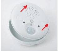
Remove the back of the housing
