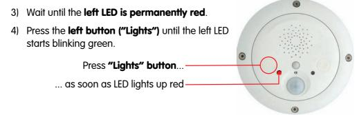
5) After several seconds, the device plays a sound twice ("Boing, Boing") and the ExtlO announces its factory default IP address via the speaker. The ExtlO is now accessible using its factory IP address (see label on the ExtlO housing).
