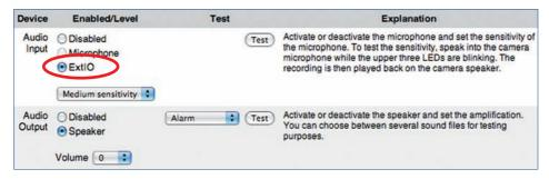
Record the voice message using the ExtlO's integrated microphone (optional: upload sound file to the camera; Admin Menu > Manage Audio Messages).
